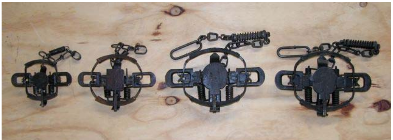
All three sizes of Victor Softcatch #1, 1 #1/12, #3 and #3 modified four-coiled matching the trap to the animal (Foot-hold traps). (Photo courtesy of Ed Carroll)
