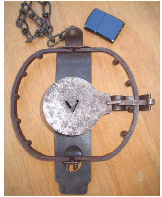
Right: Number 14 Oneida jump-trap manufactured in the 1920s–30s by the American Trap Company. They are designed for beavers and otters—the mini teeth help to grip the slippery, tough feet of the beavers. The trap has a 17.8 cm jaw spread. (Photo courtesy of Ed Carroll)
