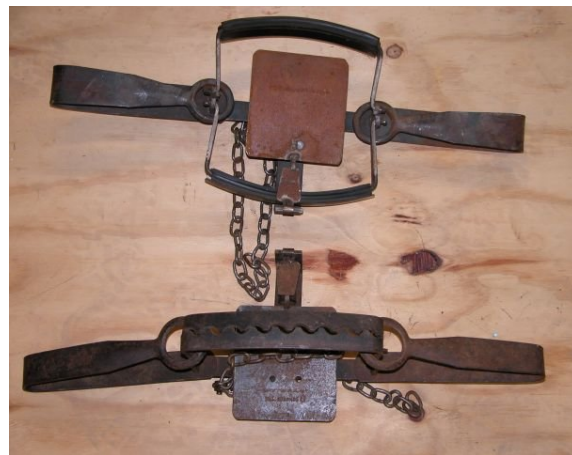
Lane's traps padded (top) and standard with teeth (bottom). Lane's traps have a 21 cm jaw spread. (Photo courtesy of Ed Carroll)
