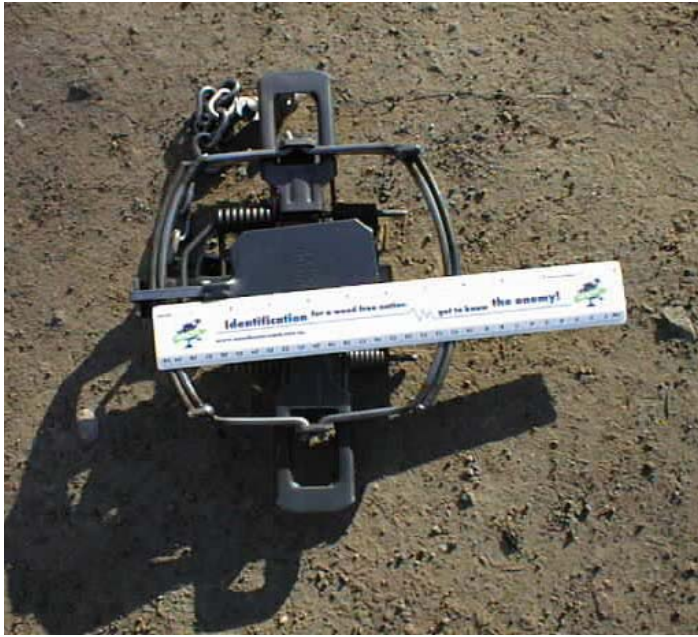
Above: Modified Bridger Number 5 laminated/offset jawed leg-hold trap, used in the United States for wolves and beavers. The trap has a 26.2 cm inside jaw spread and would be classed as a leg-hold trap for wild dogs. (Photo courtesy of Ed Carroll)
