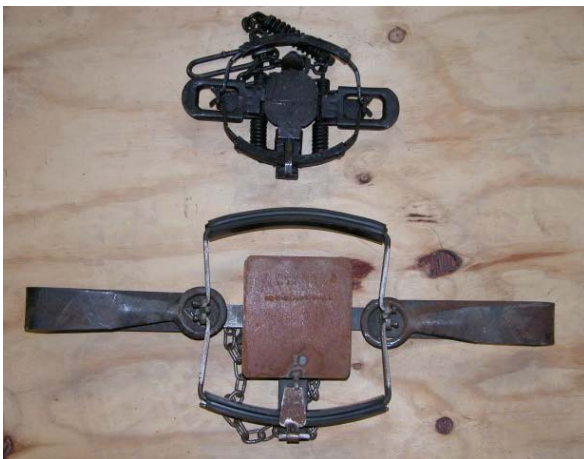
A Number 3 Victor Softcatch foot-hold trap (top) and a padded Lane's dog leg-hold trap (bottom) (Photo courtesy of Ed Carroll)
