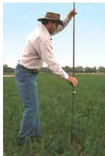
Figure 20: Using a drop penetrometer in the field to measure soil resistance
