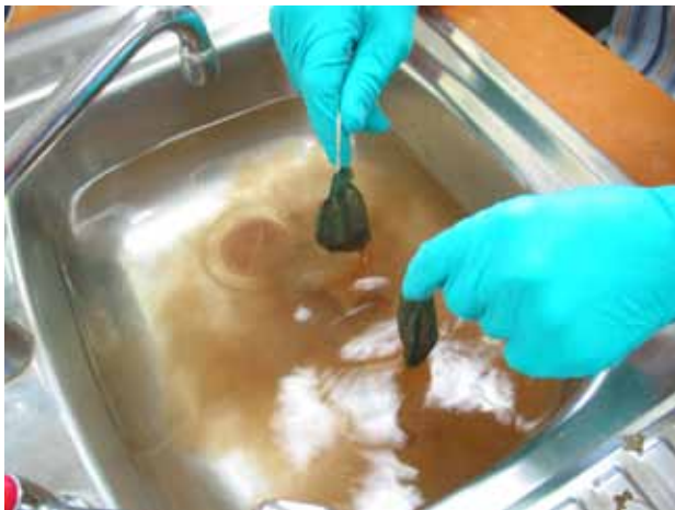
Figure 17. 20 g of sieved soil is wetted to determine its stability against the dispersal forces of water
